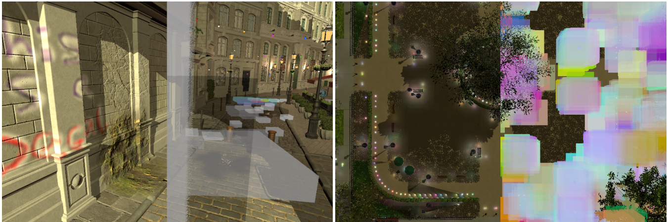
Figure 1: Left: The bistro with decals. Right: Emerald Square with 15k lights. The regions of influence are axis-aligned bounding boxes (AABBs) in an acceleration structure (right half). By tracing zero-length rays, we enumerate relevant decals and lights.
