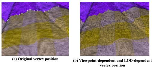
Figure 3: The viewpoint-dependent and LOD-dependent vertex position produce a blending band to eliminate the cracks.
