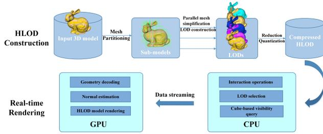
Figure 2: The pipeline of 3D viewer.
